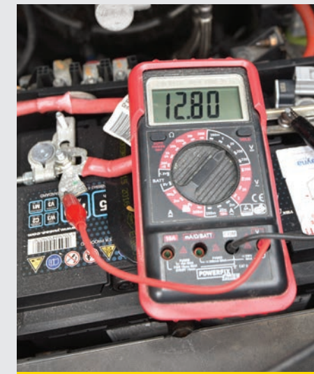
You can easily check if your charger also tops up the vehicle battery by using a multimeter set to volts – the voltage will increase when hooked up if it's receiving any charge
