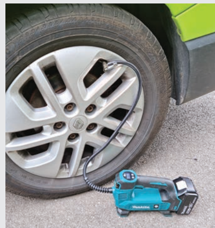
If you're not going to use the vehicle over the winter months, pump the tyres up to the maximum pressure that is stamped on the sidewalls
