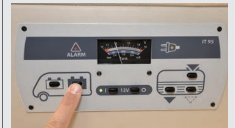
If your battery is only reading 12V, it's flat. A fully charged battery will show at least 12.8V on the panel
