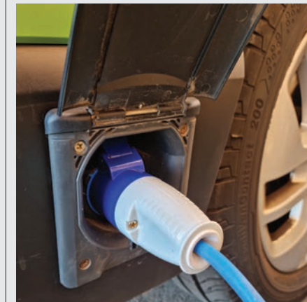
It's best to have your 'van plugged in over the winter, because solar panels are far less efficient in the cold and might not keep batteries topped up
