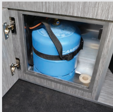
If you plan to use gas over the winter, butane (usually blue cylinders) is not the best product to use, because it doesn't work well below freezing
