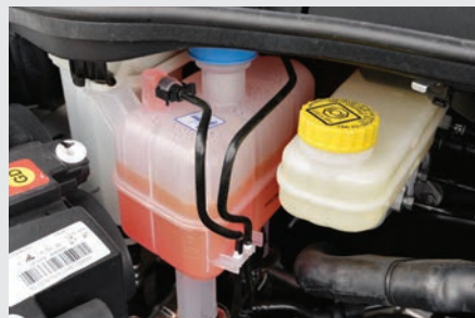
Make sure your engine coolant is not only changed at appropriate intervals, but also of the correct concentration
