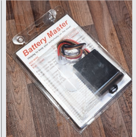
The Battery Master is a simple way to have your vehicle battery topped up automatically by the leisure batteries
