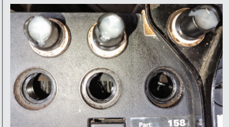
Lead plates must be immersed. If not, you'll need to add deionised water (not tap water, which will damage the cells)
