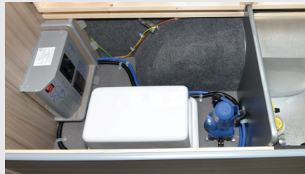
Water pumps (blue device) and hoses need to be drained down over winter
