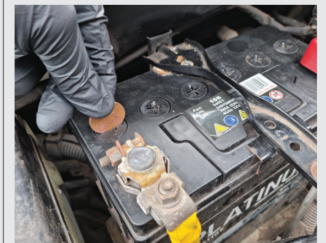
To top up the fluid in a lead acid battery, remove the cell cap with a coin. Always wear gloves and eye protection for this
