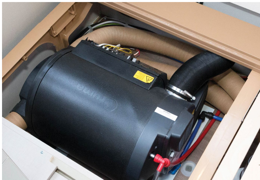
Truma's system provides blown-air heating throughout the motorhome interior
